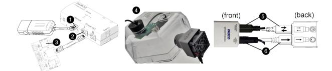
Figure 1. //control.Node, Greenhouse Sensor, and Fan Setup
