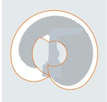
Maximum reach, maximum workspace With a reach of 600 mm and an extended workspace, the KR 4 AGILUS is ideally suited for flexible integration into compact and ultra-compact cells.
