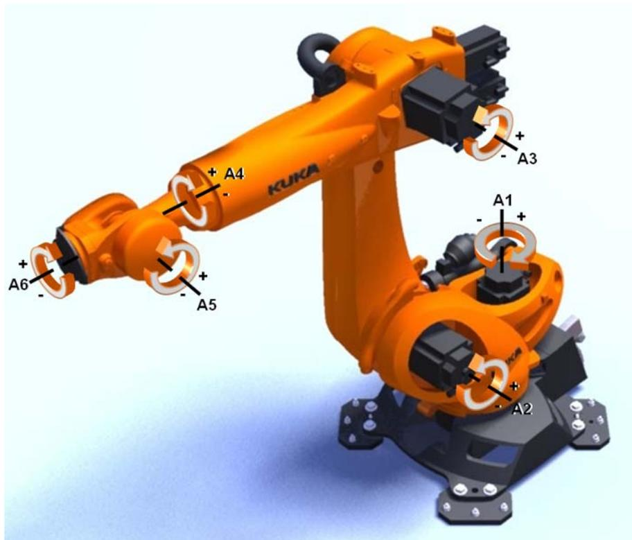
Fig. 3-4: Axes of a KUKA robot
