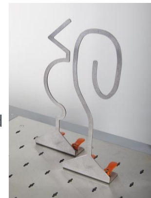
„Hot Wire“ Application For training of high precise motion. Students have to guide the eyelet through the wire contour. „Hot Wire“ Application For training of high precise motion. Students have to guide the eyelet through the wire contour.
