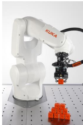
Gripper & Cubes Gripper and cubes for pick-and-place training, which are the most used robot applications.
