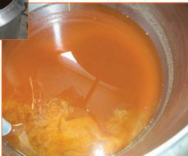
Removal of pectines : enzyming and settling
