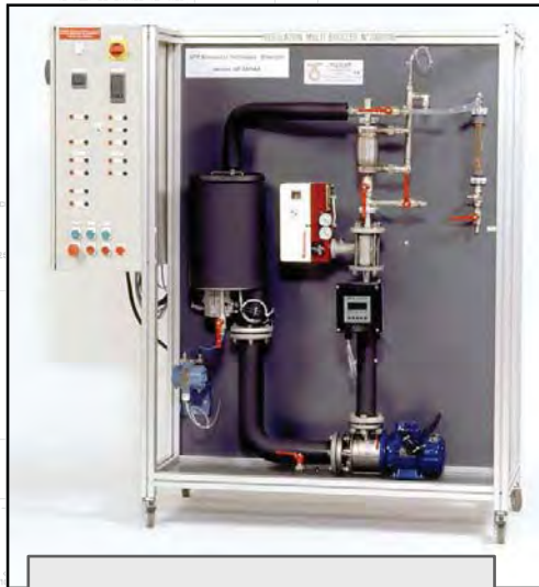
CEB1000 Multiloop regulation control Temperature, level, pressure
